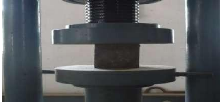
Figure1 Specimen in Compression testing Machine Table VI: Cube Compressive Strength
